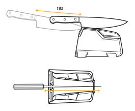
PRO TIP: For maintenance, use honing slot for weekly touch-ups.
