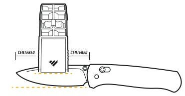
► STARTING POSITION: Note the white alignment mark on the sharpening chassis. Make sure it is pointing up. Insert the V-Block Clamp™ into the sharpening chassis so the knife handle is on the right side. This will make it easier to flip the blade over while sharpening smaller knives.
