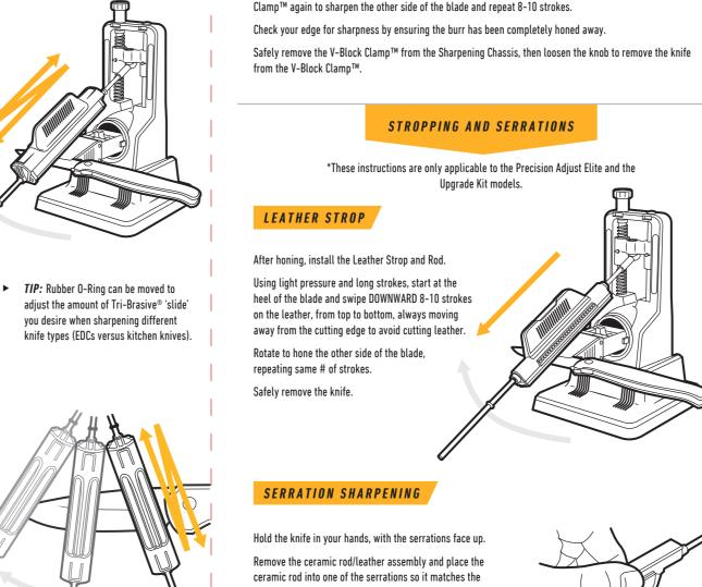
Using light pressure, swipe the ceramic rod
