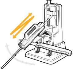
► TIP: Rubber O-Ring can be moved to adjust the amount of Tri-Brasive® 'slide' you desire when sharpening different knife types (EDCs versus kitchen knives).
