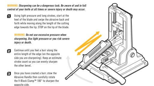
Sharpen the same number of strokes on this side of the blade to establish an even bevel.
